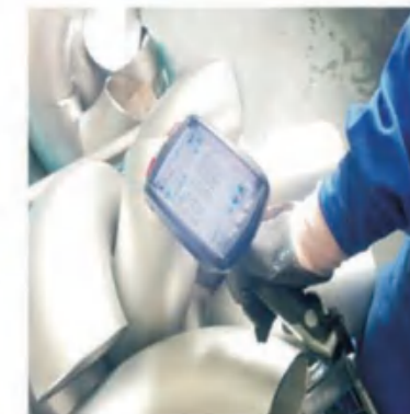
便携光谱 PMI Portable spectrometer
