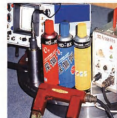
无损探伤Liquid penetrate Test
